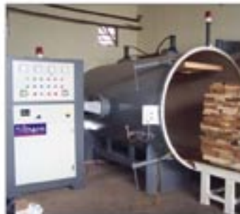
Conveyor type microwave drying in 1 to 3 hrs from MC 25% and below
