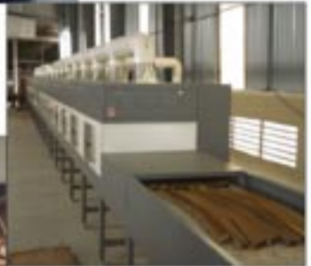
High frequency vacuum drying in 24 to 48 hrs for up to 100mm thick
