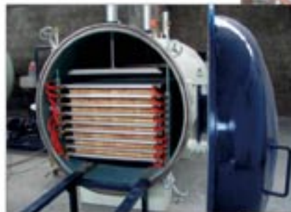
Conveyor type microwave drying in 1 to 3 hrs from MC 25% and below
