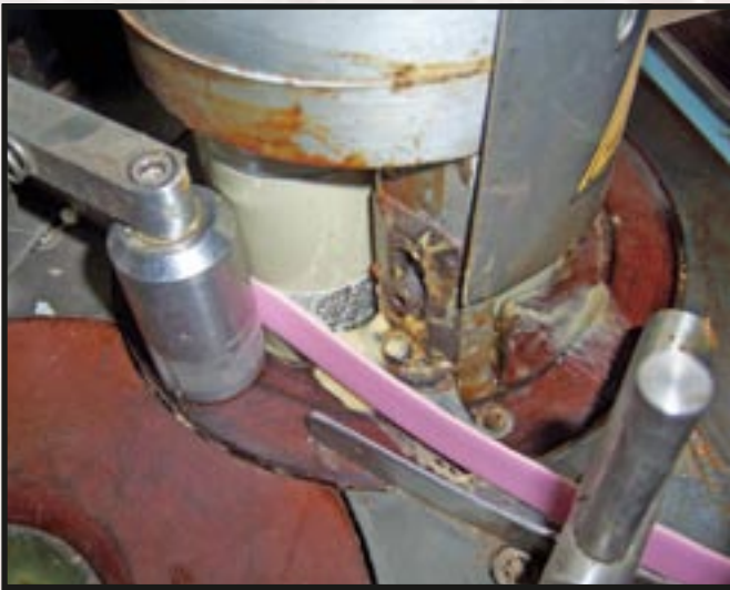
Figure 4: Hot-melt glue when the glue tank temperature is too low, resulting in stringing between the edge band and the coating roller.
