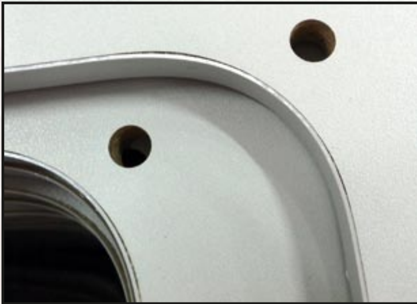
Figure 1: De-bonding on curved areas with the use of 1.00mm PVC edge band
